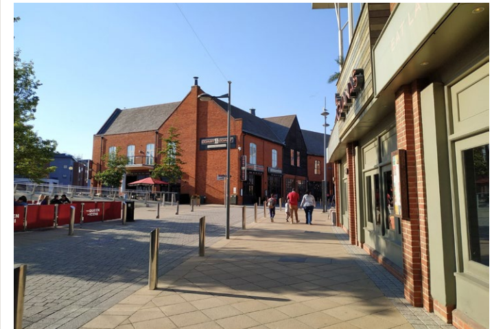
Example of lighting columns set at heights and positions to provide light to both pedestrian areas and the carriageway. It is recommended that LED lighting is used due to higher energy efficiency and power cost savings.
