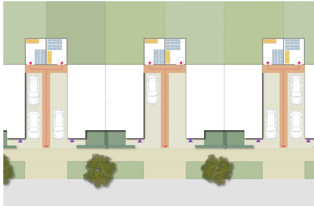
Indicative layout of a bicycle and bin storage areas at the back of properties.
