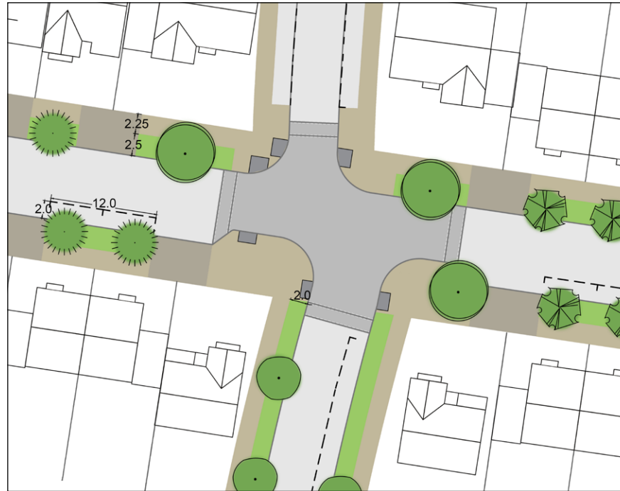
Diagram showing a typical neighbourhood junction with trees and their relationship with properties, parking spaces as well as tree-pit and verge sizes (dimensions shown in metres)
